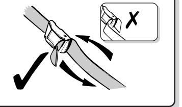
IMPORTANT: Use the red webbing straps to secure the cycle frame to the carrier. Failure to use these straps will result in the cycles falling off the carrier
